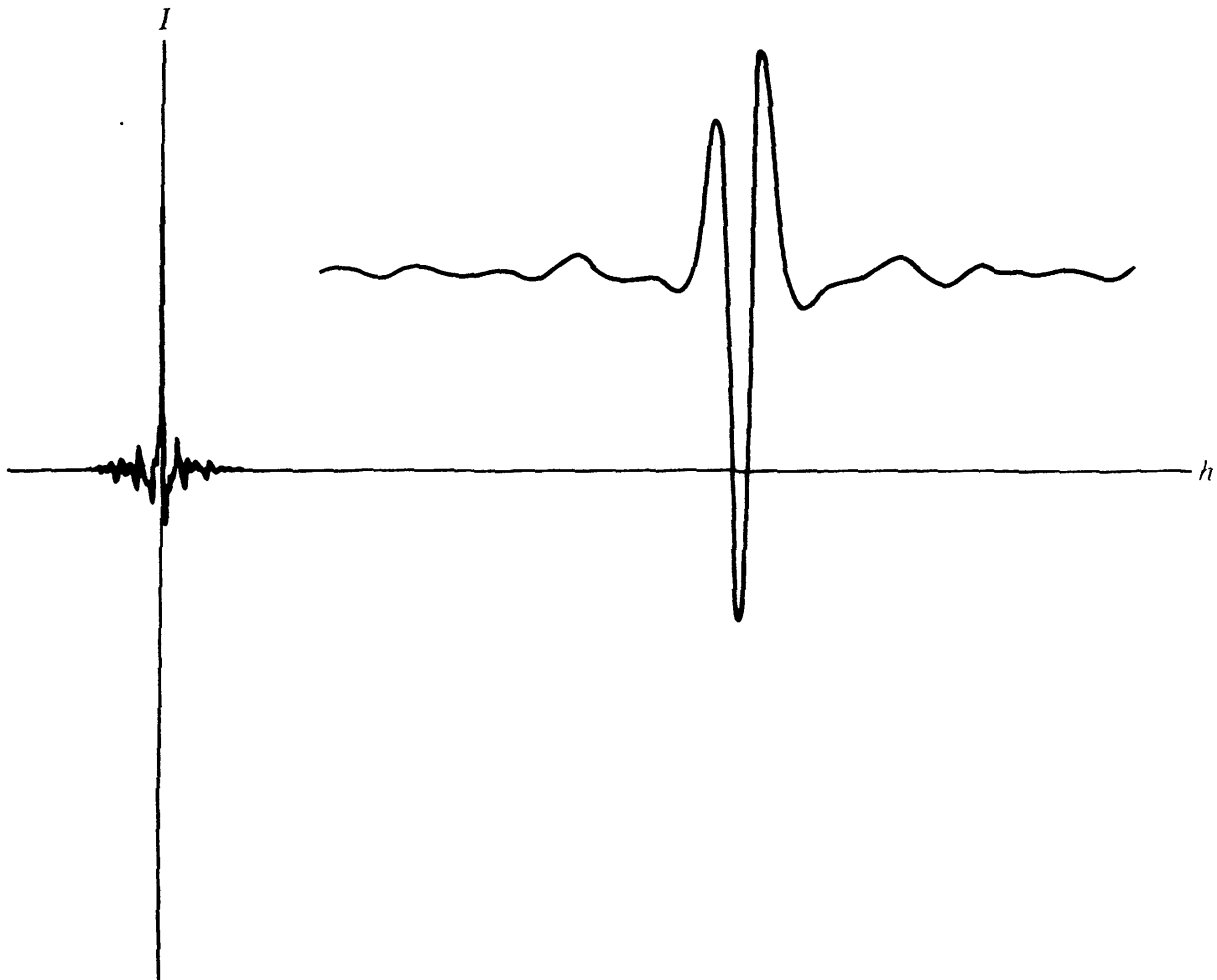
Figure 5-4. Typical midinfrared interferogram plotted with two different horizontal scales. The vertical axis represents detected intensity, and the horizontal axis represents optical path difference. The maximum optical path difference is 0.125 centimeters. (Courtesy of Peter R. Griffiths, University of California, Riverside and the American Association for the Advancement of Science. Reprinted from P. R. Griffiths, Science , vol. 222, pp. 297–302, 21 October 1983. Copyright 1983 by the American Association for the Advancement of Science.)
