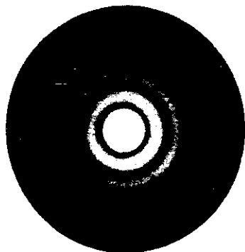
Fig. 8.12. FRAUNHOFER diffraction pattern of a circular aperture (the AIRY pattern) 6 \text{ mm} in diameter, magnification 50\times , mercury yellow light \lambda = 5790 \text{ \AA} . To show the existence of the weak subsidiary maxima, the central portion was overexposed.
