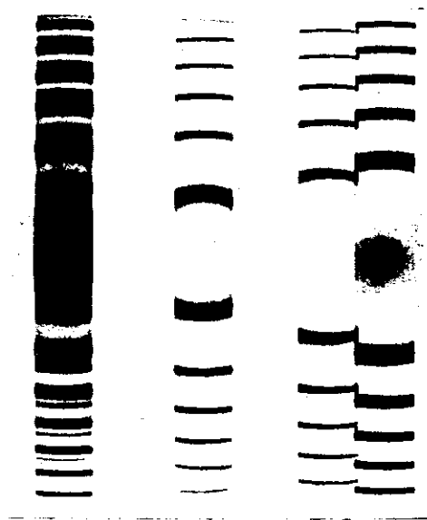
Fig. 7.64. FABRY-PEROT fringes from lines in the emission spectrum of helium (photographic negative).
