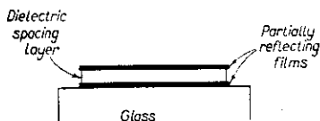
Fig. 7.71. FABRY-PEROT type interference filter.
