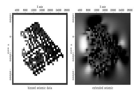
Figure 3.9: Seismic binned (left) and extended (right) by minimizing energy in  $\nabla^2 s$ . iin-misseis90 [ER]
