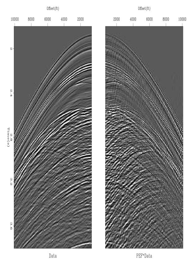
Figure 6.12: A 2-D filter (here  $20 \times 5$ ) brings out the backscattered energy. mda-antoinedecon2 [ER,M]
