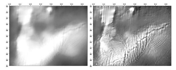
Figure 7.15: Given a PEF **A** estimated on the densely defined southern part of the model, **p** was estimated by  $\mathbf{0} \approx \mathbf{W} \frac{d}{dt} (\mathbf{L} \mathbf{A}^{-1} \mathbf{p} - \mathbf{d})$  for 50 iterations. Left is  $\mathbf{h} = \mathbf{A}^{-1} \mathbf{p}$ . Right is  $\mathbf{p} = \mathbf{H} \mathbf{h}$ . noiz-jesse9 [ER,M]
