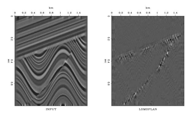
Figure 10.4: Left is a synthetic reflectivity model. Right is the result of local monoplane annihilation. Imn-sigmoid090 [ER]
