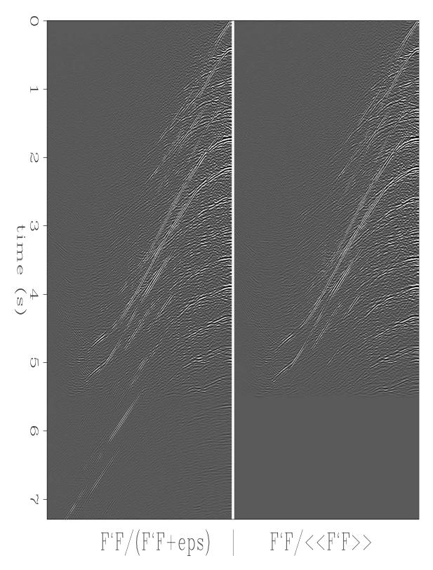
Figure 2.2: Equation (2.7) (left) and equation (2.8) (right). Both ways of dividing by zero give similar results. [Isq-antoine11] [ER]
