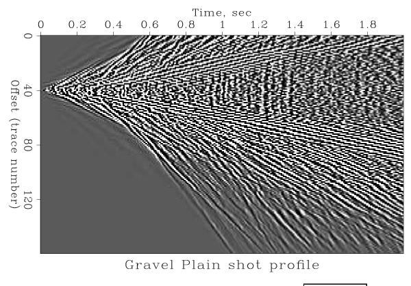
Figure 9.9: Gravel plain ground roll (Middle East) Worth testing. pch-gravel2D [ER]
