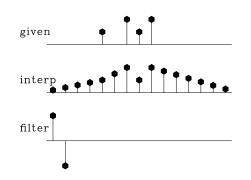
Figure 3.4: Top is the same input data as in Figure 3.3. Middle is interpolated. Bottom shows the filter (-1,2,-1). The missing data seems to be interpolated by parabolas. [iin-mparab90] [ER]
