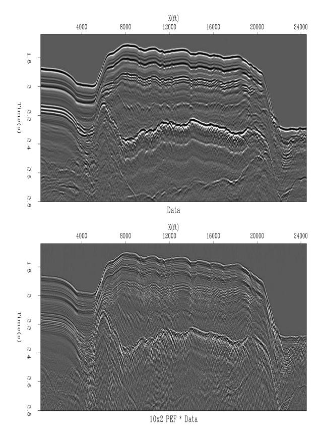
Figure 6.13: Raw data, near-trace section (top). Filtered with a two-channel PEF (bottom). The movie has other shaped filters. mda-antoinedecon3 [ER,M]
