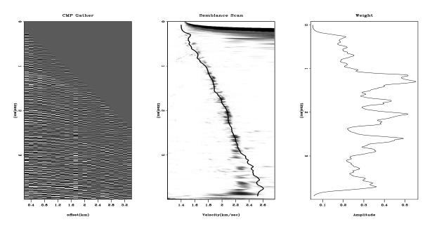
Figure 5.1: Raw CMP gather (left), Semblance scan (middle), and semblance value used for weighting function (right). (Clapp) [ER,M]
