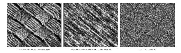
Figure 6.6: Basket weave. The simulated data fails to segregate the two dips into a checkerboard pattern. The PEF output looks structured perhaps because the filter is too small. mda-basket [ER]
