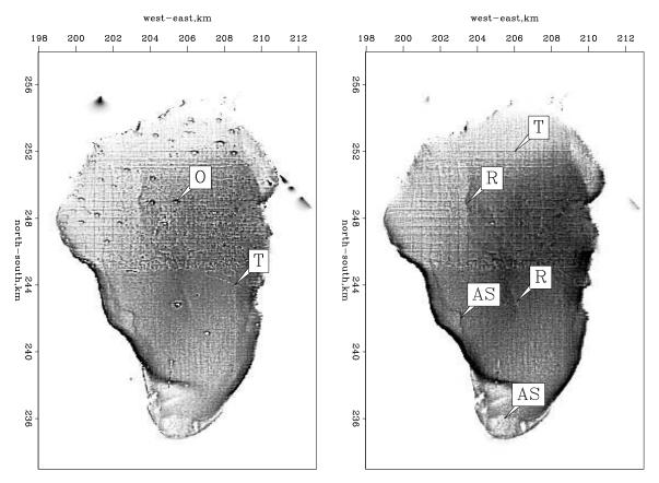
Figure 7.18: Estimated **p** in a least-squares sense (left) and in an  $\ell^1$  sense (right). Pleasingly, isolated spikes are attenuated. Some interesting features are shown by the arrows: AS points to few ancient shores, O points to some outliers, T points to few tracks, and R points to a curious feature. noiz-antoine2 [ER,M]
