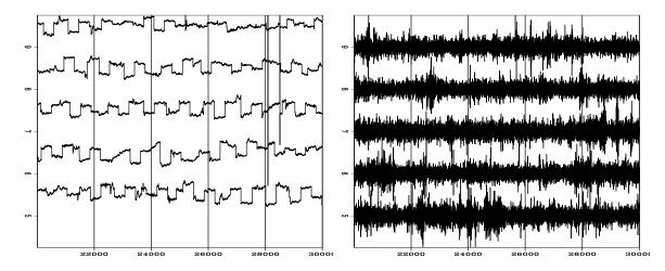
Figure 7.16: The residual at fifty thousand of the half million (537,974) data points in Figure 7.15. Left is physical residual  $\mathbf{L}\mathbf{A}^{-1}\mathbf{p} - \mathbf{d}$ . Right is fitting residual  $\mathbf{W}\frac{d}{dt}(\mathbf{L}\mathbf{A}^{-1}\mathbf{p} - \mathbf{d})$ . noiz-jesse9\_res [ER,M]
