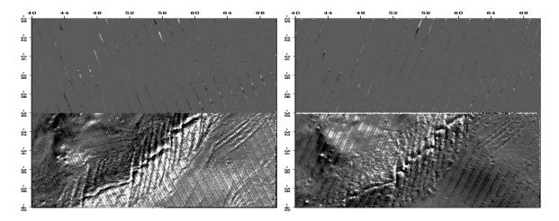
Figure 7.12: With a simple roughening derivative in data space, model space shows two nice topographic images. Let **n** denote ascending tracks. Let **s** denote descending tracks. Left is  $\mathbf{L}' \frac{d}{dt} \mathbf{n}$ . Right is  $\mathbf{L}' \frac{d}{dt} \mathbf{s}$ . [ER,M]
