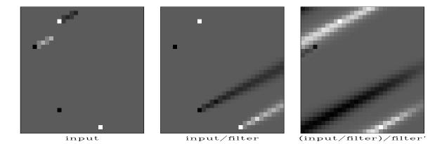
Figure 4.6: A simple low-order 2-D filter whose inverse times its inverse adjoint, is approximately a dipping seismic arrival. [hlx-dip90] [ER]
