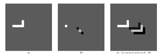
Figure 4.1: Two-dimensional convolution as performed in one dimension by module helicon [hlx-diamond90] [ER]
