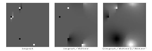
Figure 4.8: Deconvolution by a filter whose autocorrelation is the two-dimensional Laplacian operator. Amounts to solving the Poisson equation. Left is q; Middle is  $q/\mathcal{H}$ ; Right is  $(q/\mathcal{H})/\mathcal{H}'$ . [hlx-lapfac90] [ER]
