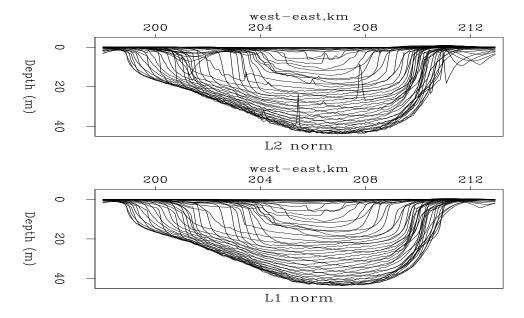
Figure 7.19: East-west cross sections of the lake bottom ( $\mathbf{h} = \mathbf{H}^{-1}\mathbf{p}$ ). Top with the  $\ell^2$  solution. Bottom with the  $\ell^1$  approximating procedure. noiz-antoine3 [ER,M]
