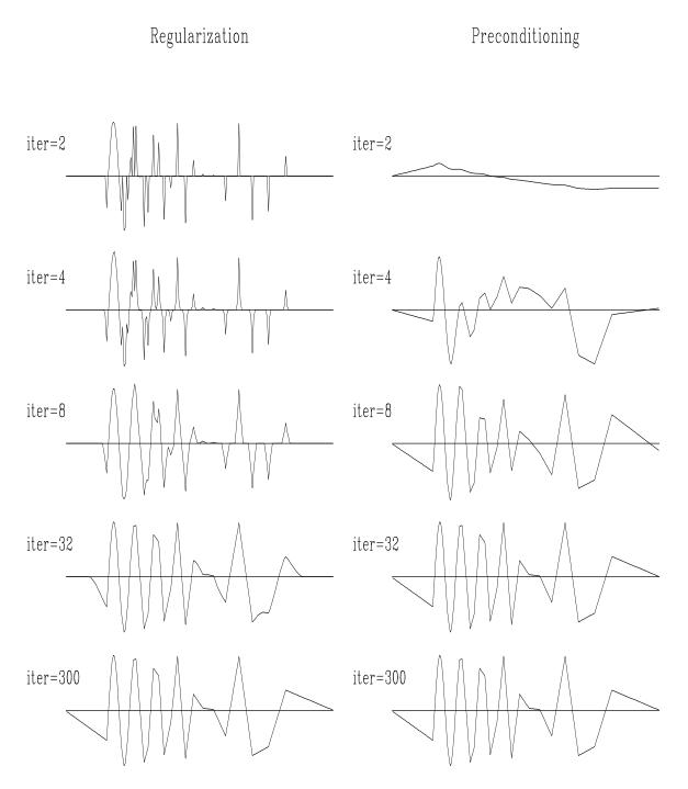
Figure 5.6: Convergence history of inverse linear interpolation. Left: regularization, right: preconditioning. The regularization operator **A** is the derivative operator (convolution with (1, -1)). The preconditioning operator **S** is causal integration. prc-conv1 [ER,M]
