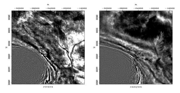
Figure 11.1: Some time slices show a salt dome, some river channels, a dendritic drainage canyon, and a fault. Press button for interactive "Rickmovie". [rez-canyon] [ER]
