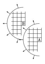
Figure 6.2 shows the input plane with a 2-D filter on top of it at two possible locations. The filter shape is a semidisk, which you should imagine being of infinitely large radius. Notice that semidisk A includes all the points in B. The output of disk A will be shown to be orthogonal to the output of disk B. Conventional least squares theory says that the coefficients of the filter are designed so that the output of the filter is orthogonal to each of the inputs to
