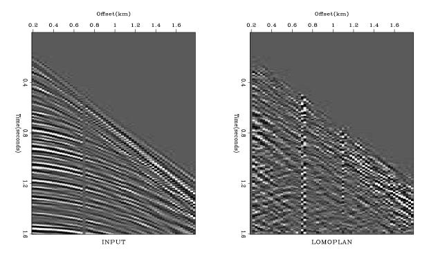
Figure 10.7: Portion of Yilmaz and Cumro data set 27 (left) and after LOMOPLAN (right). Press button for movie. Imn-yc2790 [ER]
