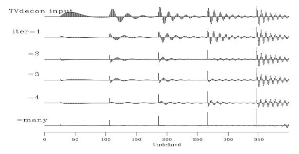
Figure 9.15: Time variable deconvolution with two free filter coefficients and a gap of 6. pch-tvdecon90 [ER]
