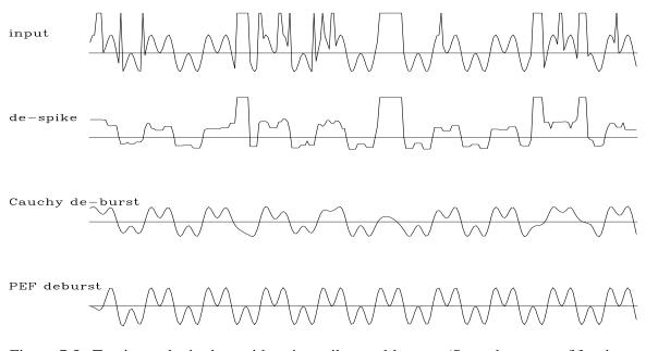
Figure 7.5: Top is synthetic data with noise spikes and bursts. (Some bursts are fifty times larger than shown.) Next is after running medians. Next is Laplacian filter Cauchy deburst processing. Last is PEF-deburst processing. noiz-pefdeburst90 [ER]
