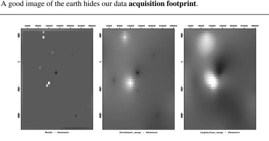
Figure 3.11: Difference between wells (the final map) and the extended seismic data. Left is plotted at the wells (with gray background for zero). Center is based on gradient roughening and shows tent-pole-like residuals at wells. Right is based on Laplacian roughening. iin-diffdiff90 [ER]
