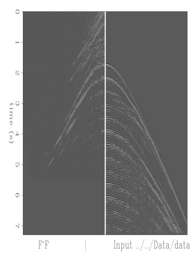
Figure 2.1: 2-D data (right) and a quadrant of its autocorrelation (left). Notice the longest nonzero time lag on the data is about 5.5 sec which is the latest nonzero signal on the autocorrelation. Isq-antoine10 [ER]
