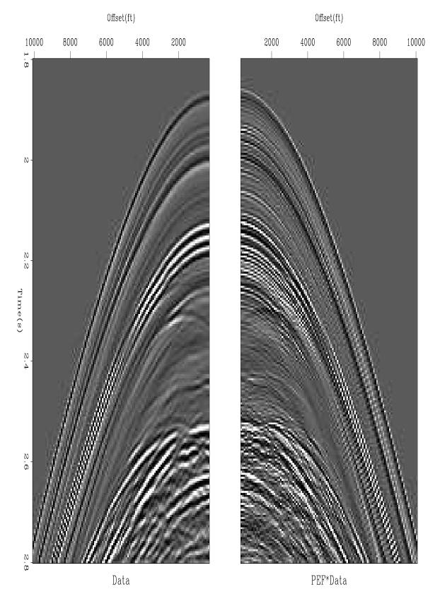
Figure 6.11: Raw data with its mirror. Mirror had 1-D PEF applied, 30 point filter. mda-antoinedecon [ER,M]
