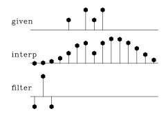
Figure 3.5: Top is the same input. Middle is interpolated. Bottom shows the filter (1, -3, 3, -1). The missing data is very smooth. It shoots upward high off the right end of the observations, apparently to match the data slope there. iin-mseis90 [ER]
