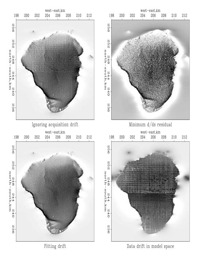
Figure 7.20: Top left: Estimated **p** without attenuation of the tracks, i.e., regression (7.23). Top right: Estimated **p** with the derivative along the tracks, i.e., regression (7.25). Bottom left: Estimated **p** without tracks, i.e., regression (7.26). Bottom right: recorder drift in model space **B'Lq**. noiz-antoine4 [ER,M]
