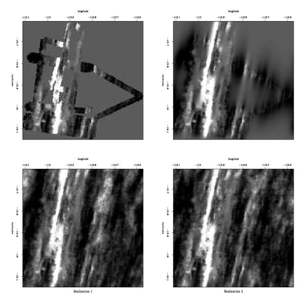
Figure 6.20: Top left is binned data. Top right extends the data with a PEF. The bottom two panels add appropriately colored random noise in the regions of missing data. [mda-bobsea] [ER,M]
