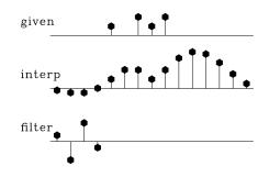
Figure 3.6: Bottom shows the filter (1, 1). The interpolation is rough. Like the given data itself, the interpolation has much energy at the Nyquist frequency. But unlike the given data, it has little zero-frequency energy. iin-moscil90 [ER]
