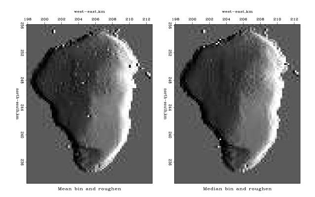
Figure 7.4: Galilee water depth binned and roughened. Left is binning with the mean, right with the median. noiz-medbin90 [ER,M]
