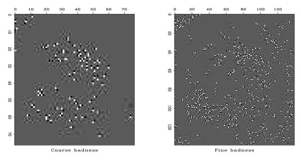
Figure 2.6: Values of curl at Vesuvius. The bad data locations at both coarse and fine resolution tend to occur in pairs of opposite polarity. [Isq-screw90] [ER,M]
