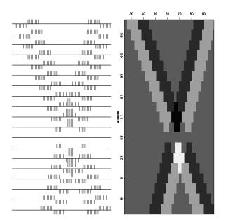
Figure 10.3: Superposition of plane waves of opposite polarity. Imn-super90 [ER]
