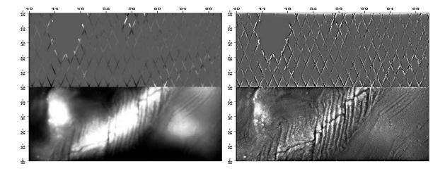
Figure 7.13: All data merged into a track-free image (hooray!) by applying the track derivative, not to the data, but to the residual. Left is **h** estimated by  $\mathbf{0} \approx \mathbf{W} \frac{d}{dt} (\mathbf{L}\mathbf{h} - \mathbf{d})$ . Right is the roughened altitude,  $\mathbf{p} = \mathbf{H}\mathbf{h}$ . noiz-jesse10 [ER,M]
