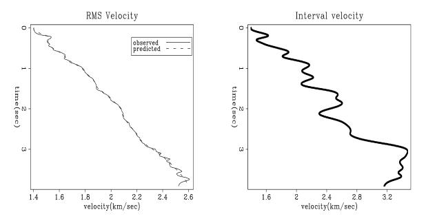
Figure 5.3: Observed RMS velocity and that predicted by a flexible model with  $\epsilon = .25$  (Clapp) prc-flex [ER]
