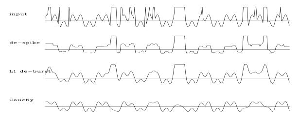
Figure 7.3: Top is synthetic data with noise spikes and bursts. (Most bursts are a hundred times larger than shown.) Next is after running medians. Bottom is after the two processes described here. noiz-burst90 [ER]
