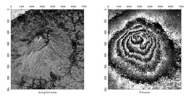
Figure 2.4: Radar image of Mt. Vesuvius. Left is the amplitude. Non-reflecting ocean in upper left corner. Right is the phase. (Umberto Spagnolini) Isq-vesuvio90 [ER,M]
