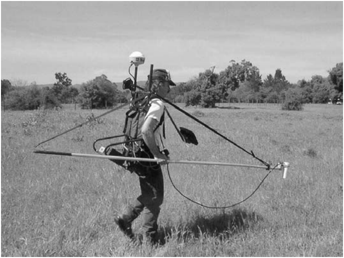
Figure 1.11 Magnetometer coupled to a differential GPS navigation system. Unless allowance is made in processing for the offset between the GPS aerial (behind the operator's head) and the magnetometer sensor (at the end of the horizontal bar), anomalies will be incorrectly located on detailed maps (photo courtesy Geometrics Inc.)
