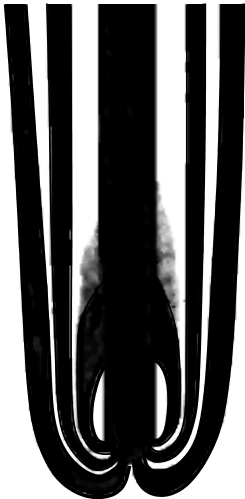
Fig. 9.5. Differential interferogram of the vertical heated plate, \text{Gr}_z = 8 \cdot 10^6
