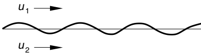
Fig. 10.30. Stability of an interface between two layered fluids, velocity of the phases u_1, u_2
