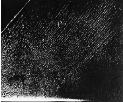
Fig. 8.9. Decay of cross-flow instability into a three-dimensional boundary layer, Kohama (1989)
