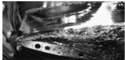
bubble cavitation, Re = 10^6, \sigma = 0.08
