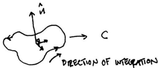
Figure 3: Direction convention for integration around a closed contour, C . The vector \hat{\mathbf{n}} is the unit normal to the surface.
