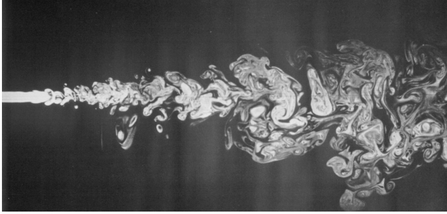
Figure 1: The scalar concentration of a turbulent water jet.
