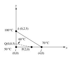
Figure 3.8 Isotherm within a linear triangular element
