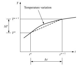
Figure 6.3 Temperature variation within a time step
