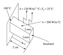
Figure 3.29 Heat transfer from a rectangular fin
