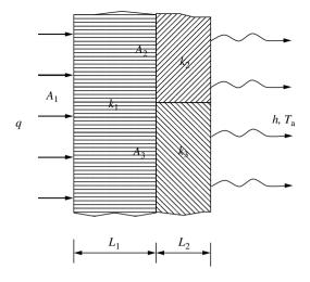
Figure 2.9 Heat transfer in a composite wall
