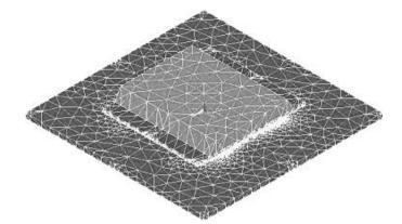
Figure 9.26 Element model of PBGA
