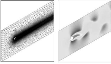
(a) Finite element surface mesh
