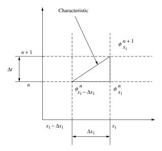
Figure 7.8 Characteristic in a space-time domain
