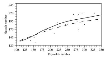
Figure 8.5 Forced convection in a channel. Comparison of the Nusselt number with experimental data for different particle Reynolds numbers. Points—experimental (Vafai *et al.* 1984); dashed line—numerical (Vafai *et al.* 1984); solid—CBS
