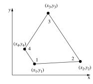
Figure 3.13 A typical quadrilateral element
