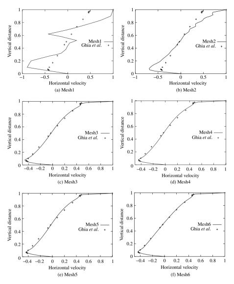
Figure 9.5 Incompressible isothermal flow in a lid-driven cavity.  $u_1$  velocity profile along the mid-vertical line. Comparison with the benchmark steady state results of Ghia *et al.* (Ghia *et al.* 1982)
