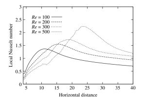
Figure 9.23 Forced convection heat transfer downstream of a backward-facing step. Local Nusselt number distribution on the hot wall for different Reynolds numbers
