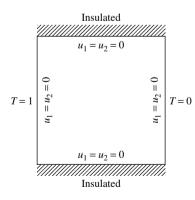
Figure 7.26 Buoyancy-driven flow in a square enclosure. Geometry and boundary conditions
