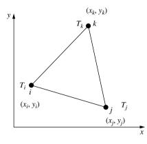
Figure 3.7 A linear triangular element
