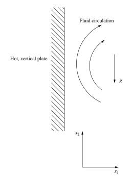
Figure 7.7 Natural convective flow near a hot, vertical plate
