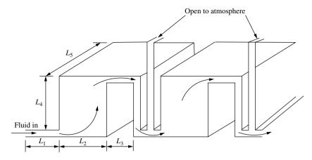
Figure 9.38 Schematic diagram of water processing plant, inlet/exit channel height = 1,  $L_1 = 4$ ,  $L_2 = 5$ ,  $L_3 = 4$ ,  $L_4 = 6$ ,  $L_5 = 30$
