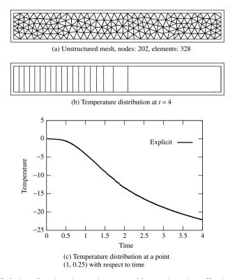
Figure 6.15 Solution for the phase change problem using the effective heat capacity method
