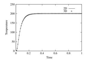
Figure 6.12 Temperature distribution at the centre of a square domain (cube in 3D) with respect to time
