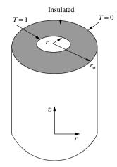
Figure 8.10 Natural convection in a fluid-saturated constant porosity medium. Problem definition
