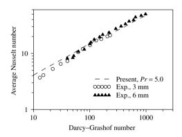
Figure 8.11 Natural convection in a fluid-saturated constant porosity medium within an annular enclosure. Comparison of hot wall steady state Nusselt number with the experimental and numerical data (Prasad *et al.* 1985)
