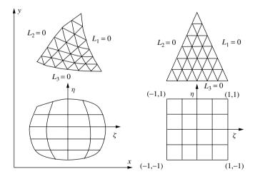
Figure 3.17 Isoparametric mapping of triangles and quadrilaterals
