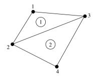
Figure C.1 A domain with two linear triangular elements
