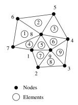
Figure 10.1 A typical unstructured mesh
