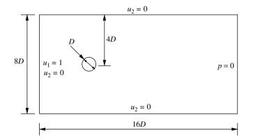
Figure 9.16 Isothermal flow past a circular cylinder. Geometry and boundary conditions
