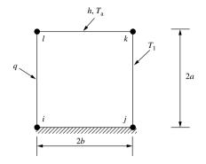
Figure 5.11 Rectangular element with different boundary conditions
