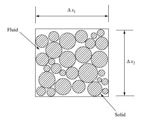
Figure 8.3 Fluid-saturated porous medium. Infinitesimal control volume
