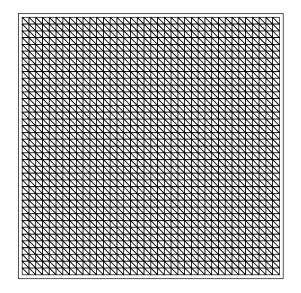
Figure 5.7 Fine structured mesh
