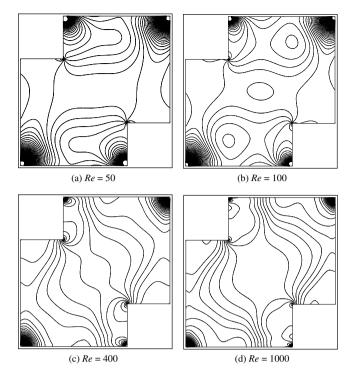
Figure 9.14 Incompressible isothermal flow in a double-driven cavity. Pressure contours for different Reynolds numbers
