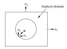
Figure 10.4 Multiply connected domain. Outward normal
