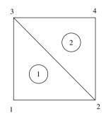
Figure 5.10 Discretization using two triangular elements
