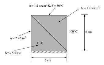
Figure 5.9 A square domain with mixed boundary conditions
