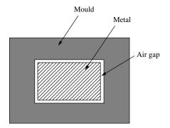
Figure 2.13 Casting and mould arrangement
