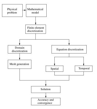
Figure 3.1 Numerical model for heat transfer calculations
