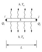
Figure 2.5 A typical element from the rectangular fin arrangement and conductive-convective heat transfer mechanism
