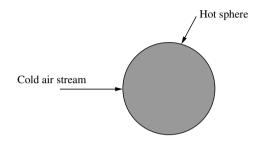
Figure 7.22 Forced convection flow past a sphere
