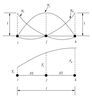
Figure 3.5 Variation of shape functions and their derivatives over a one-dimensional quadratic element
