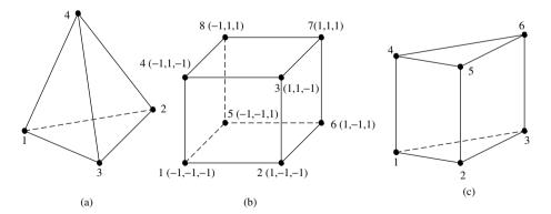
Figure 3.21 Three-dimensional elements, (a) tetrahedron, (b) hexahedron and (c) prism
