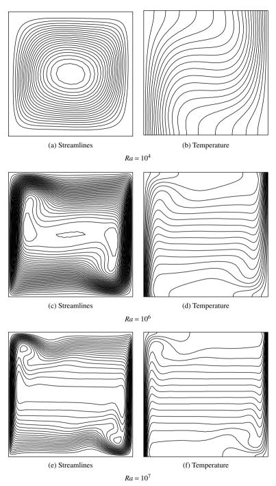
Figure 7.28 Natural convection in a square enclosure. Streamlines and temperature contours for different Rayleigh numbers, Pr = 0.71
