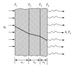
Figure 4.2 Heat conduction in a composite wall
