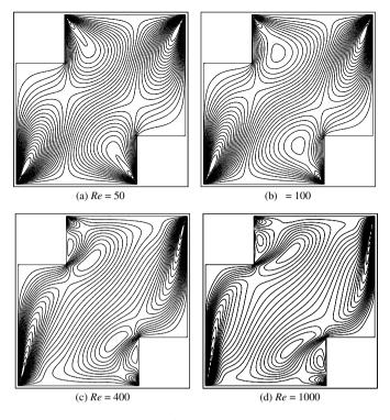
Figure 9.13 Incompressible isothermal flow in a double-driven cavity.  $u_2$  velocity contours for different Reynolds numbers
