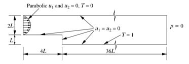
Figure 9.19 Forced convection heat transfer downstream of a backward-facing step. Geometry and boundary conditions
