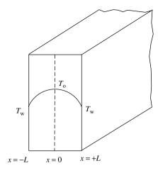
Figure 4.6 Plane wall with heat source
