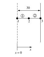
Figure 4.9 Quadratic finite element discretization
