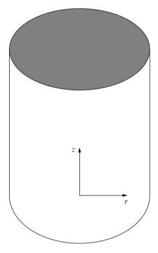
Figure 7.35 Coordinate system for axisymmetric geometries
