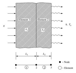
Figure 2.1 Heat transfer through a composite slab
