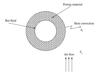
Figure 7.14 Example of convection boundary condition
