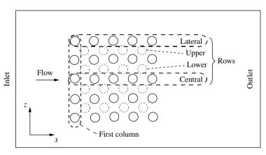
(b) Staggered arrangement and rows and column names
