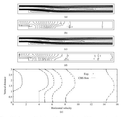
Figure 9.10 Incompressible isothermal flow past a backward-facing step. (a)  $u_1$  velocity contours (mesh1), (b) pressure contours (mesh1), (c)  $u_1$  velocity contours (mesh2), (d) pressure contours (mesh2) and (e) comparison of velocity profiles with experimental data (mesh1), Re = 229
