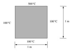
Figure 5.4 Square plate with different temperature boundary conditions
