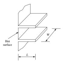
Figure 2.3 Array of thin rectangular fins
