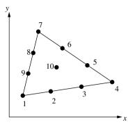
Figure 3.12 Ten-node cubic triangular element
