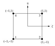
Figure 3.15 Non-dimensional coordinates of a rectangular element
