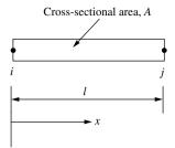
Figure 6.2 One-dimensional linear element
