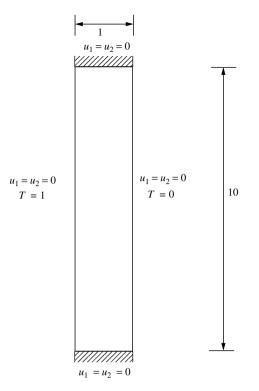
Figure 8.7 Natural convection in a fluid-saturated variable porosity medium. Problem boundary conditions
