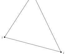
Figure 7.12 Two-dimensional linear triangular element
