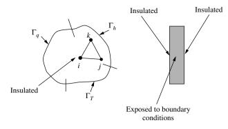
Figure 5.2 Typical two-dimensional plane geometry and triangular element
