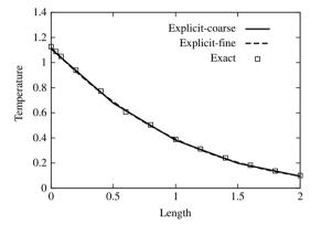
Figure 6.8 Temperature distribution along the length of the rod at t = 1
