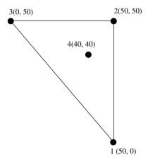
Figure 5.8 Interpolation into a triangular element
