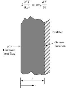
Figure 6.16 Heat conduction through a wall. Inverse problem
