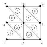
Figure 5.5 Discretization using triangular elements
