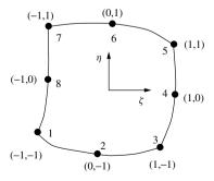
Figure 3.18 Eight-node isoparametric element
