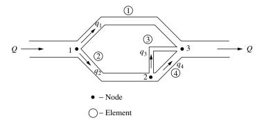
Figure 2.2 Fluid flow network
