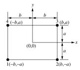
Figure 3.14 A simple rectangular element
