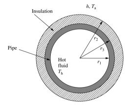
Figure 2.10 Heat transfer through an insulating material
