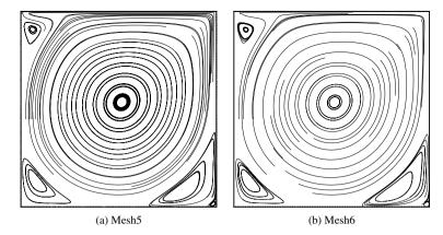
Figure 9.4 Isothermal flow in a lid-driven cavity. Stream traces at Re = 5000
