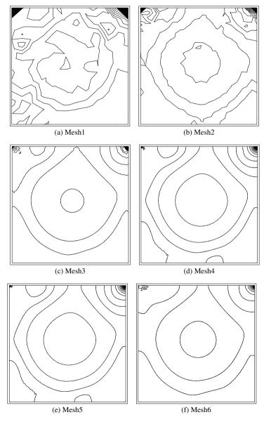
Figure 9.3 Isothermal flow in a lid-driven cavity. Pressure contours at Re = 5000
