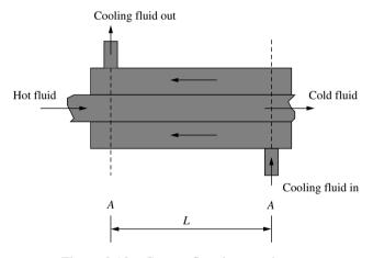
Figure 2.12 Counterflow heat exchanger
