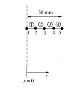
Figure 4.7 Finite element discretization
