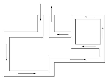
Figure 2.11 Pipe network for central heating
