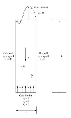
Figure 7.29 Mixed convection in a vertical channel. Geometry and boundary conditions
