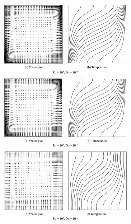
Figure 8.9 Natural convection in a fluid-saturated porous, square enclosure. Vector plots and temperature contours for different Rayleigh and Darcy numbers; Pr = 0.71
