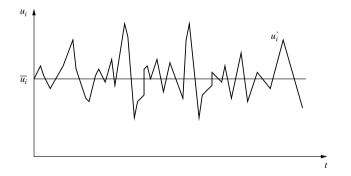
Figure 7.33 Turbulence velocity variation with time
