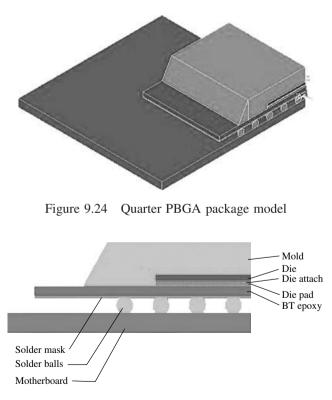
Figure 9.25 Detailed model of PBGA
