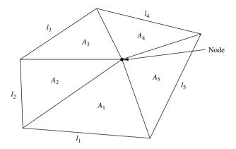
Figure 7.13 Two-dimensional linear triangular element
