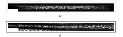
Figure 9.9 Incompressible isothermal flow past a backward-facing step. Finite element meshes. (a) Nodes:4656, elements:8662, (b) nodes:3818, elements:7155
