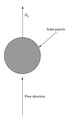
Figure 8.1 Drag force on a porous medium grain
