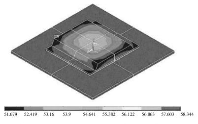
Figure 9.28 Temperature distribution of expanded full model
