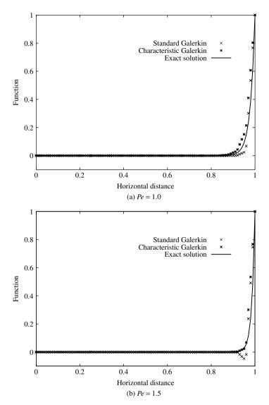
Figure 7.11 Spatial variation of a function,  $\phi$ , in one-dimensional space for different element Peclet numbers
