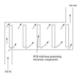
Figure 2.17 Assembly of printed circuit boards
