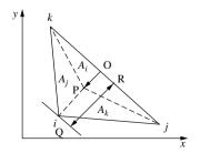
Figure 3.9 Area coordinates of a triangular element
