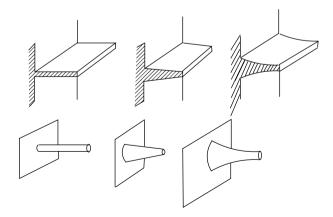
Figure 4.12 Different types of fins
