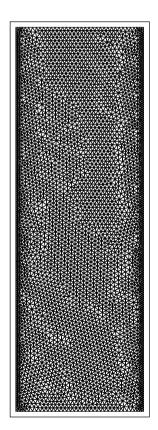
Figure 7.30 Mixed convection in a vertical channel. Unstructured finite element mesh
