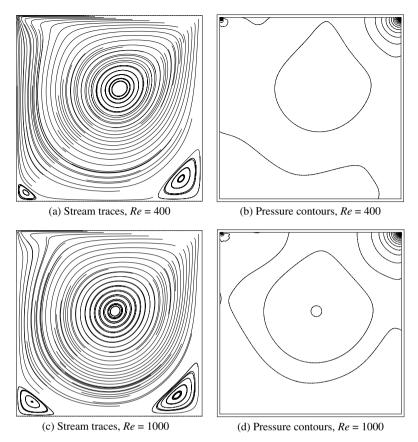
Figure 9.6 Isothermal flow in a lid-driven cavity. Stream traces and pressure contours for different Reynolds numbers
