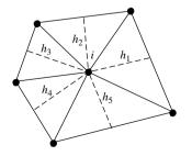
Figure 10.5 Element size calculation
