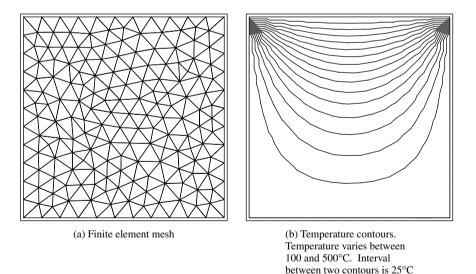
Figure 5.6 Solution for Example 5.2.1 on an unstructured mesh. The temperature obtained at the centre of the plate is  $200.42 \,^{\circ}\text{C}$
