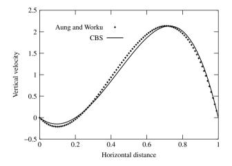
Figure 7.32 Mixed convection in a vertical channel. Comparison of velocity profile at exit with fully developed analytical solution (Aung and Worku 1986b)
