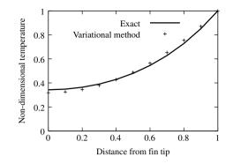
Figure 3.26 Comparison between variational method and exact solution
