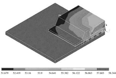
Figure 9.27 Temperature distribution of quarter PBGA model
