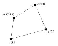
Figure 3.32 Quadrilateral element
