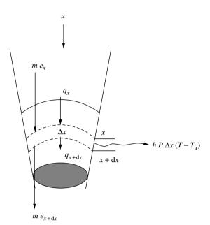
Figure 1.3 Conservation of energy in a moving body
