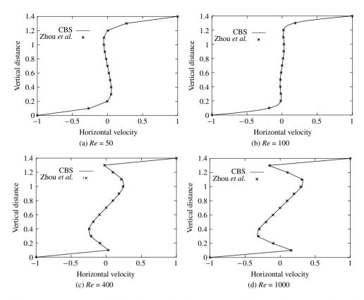
Figure 9.15 Incompressible isothermal flow in a double-driven cavity. Comparison of horizontal velocity profile at mid-vertical section with Zhou *et al.* (Zhou *et al.* 2003) for different Reynolds numbers
