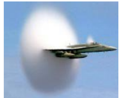
ab / This fighter jet has just accelerated past the speed of sound. The sudden decompression of the air causes water droplets to condense, forming a cloud.
