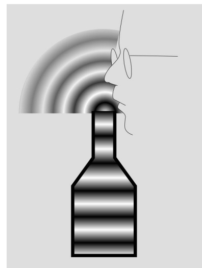
v / Surprisingly, sound waves undergo partial reflection at the open ends of tubes as well as closed ones.
