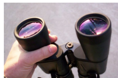
j / Seen from this angle, the optical coating on the lenses of these binoculars appears purple and green. (The color varies depending on the angle from which the coating is viewed, and the angle varies across the faces of the lenses because of their curvature.)
