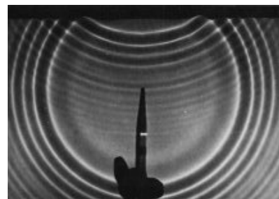
a / Circular water waves are reflected from a boundary on the left.
