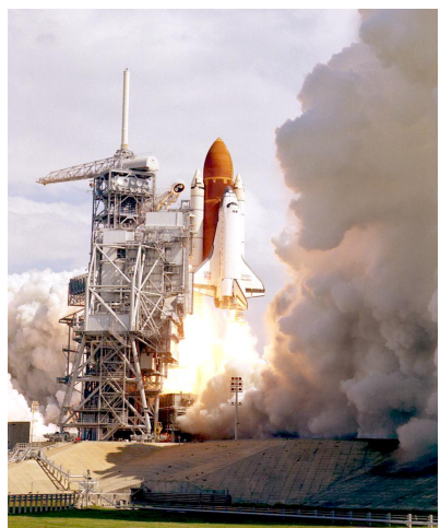
c / Rockets work by pushing exhaust gases out the back. Newton's third law says that if the rocket exerts a backward force on the gases, the gases must make an equal forward force on the rocket. Rocket engines can function above the atmosphere, unlike propellers and jets, which work by pushing against the surrounding air.
