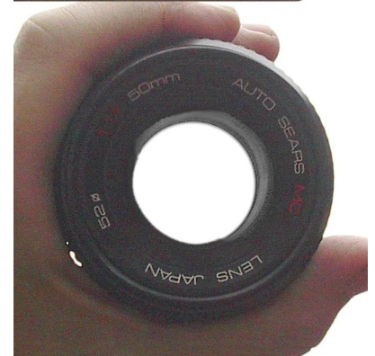
d/The same lens is shown with its diaphragm set to three different apertures.
