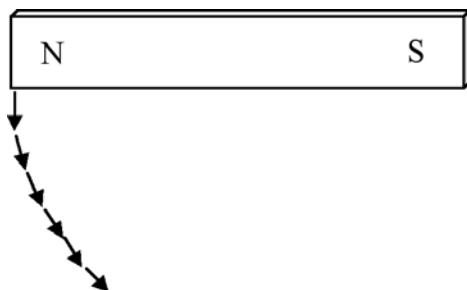
Figure 4 Constructing magnetic field lines
