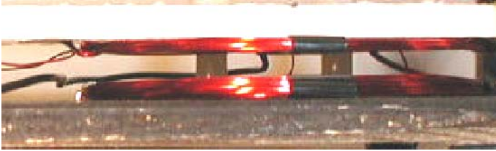
Figure 5 Spacing between the 10-turn and 38-turn coils
