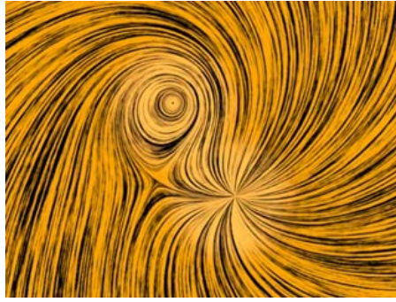
Figure 1.4.8 A flow field that has both a source (divergence) and a circulation (curl).
