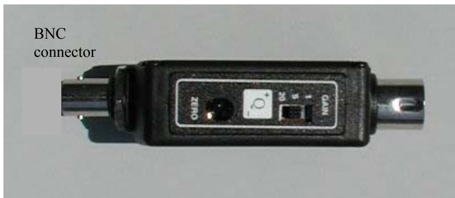
Figure 5 Gain and Zero Settings for Charge Sensor.
