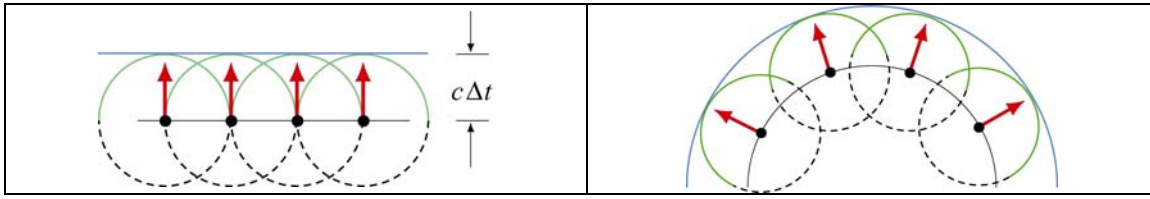
Figure 14.4.1 Propagation of wave based on Huygens's principle.
