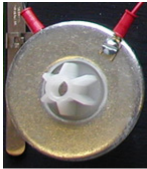
Figure 1 Perf-board used as spacers on washer
