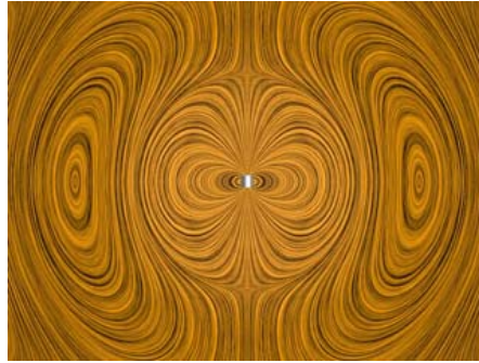
Figure 13.8.6 Radiation from an electric dipole whose dipole moment completely reverses with time.
