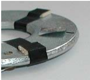
Figure 2 Charge flows to edge of foil
