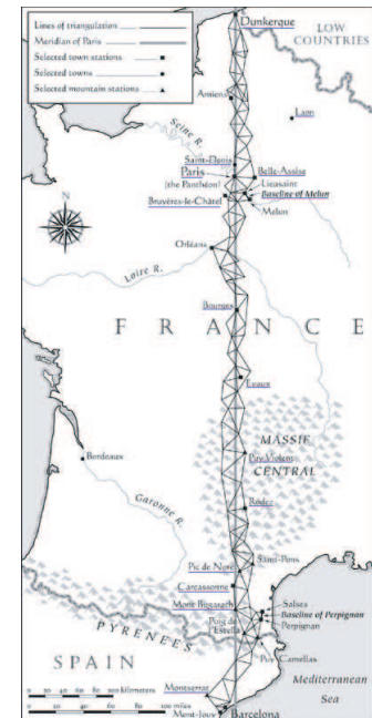
FIGURE 65 The measurements that lead to the definition of the metre (© Ken Alder)
